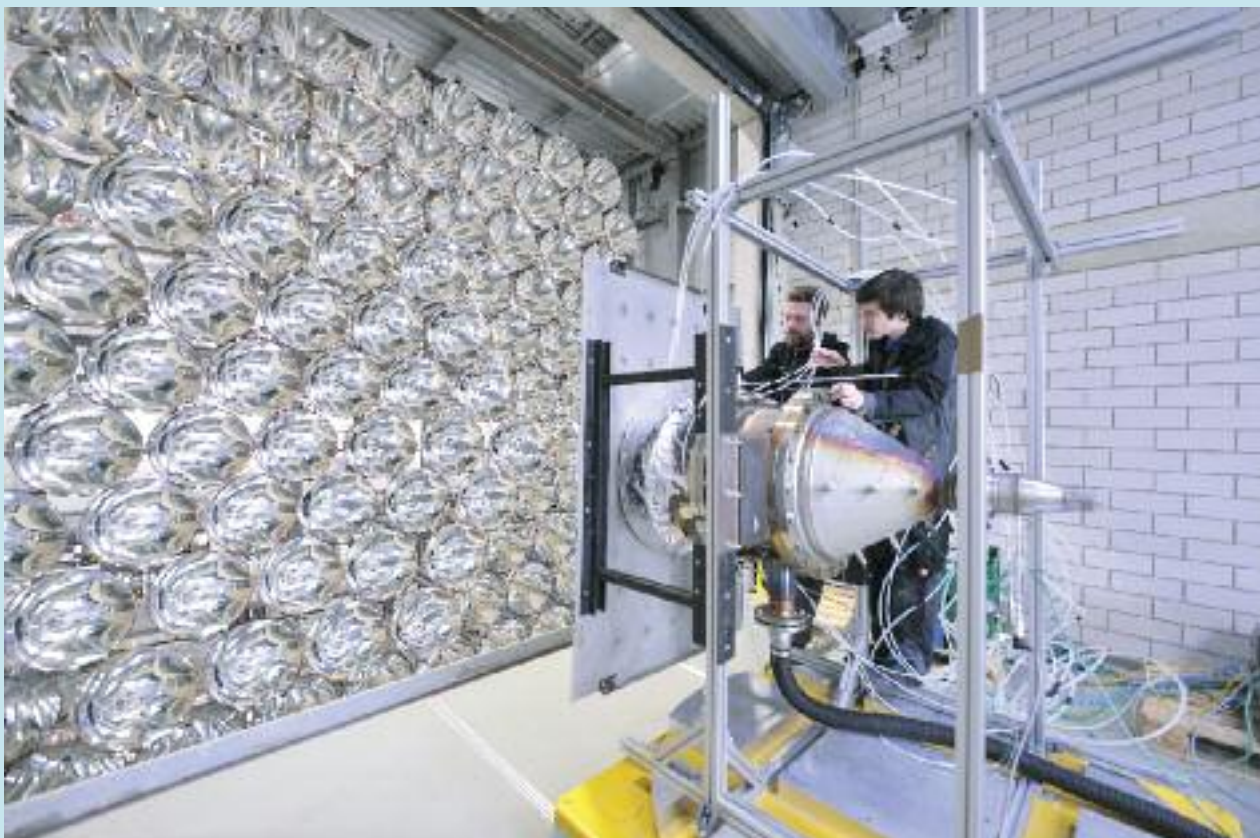
The 149 lamps that make up the artificial sun form a wall 16 meters high and concentrate their light on a single point, where the reactor used to generate hydrogen is located (photo above).
