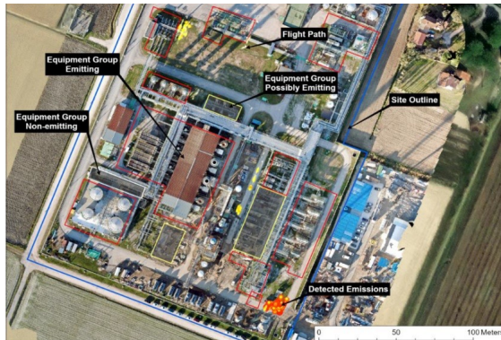
Figure 2 - Source level vs. site level reconciliation
