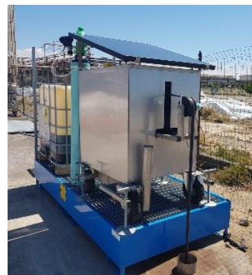
Figure 8-2: The e-hyrec® device positioned in the water table. It comprises the part lowered into the well and the handling, management and control system located on the well's mouth.
