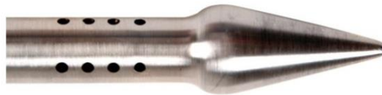
Figure 8-9: Stainless steel probe with the polyethylene film inside for field installation through direct push techniques
