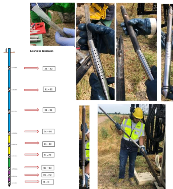
Figure 8-11: Passive sampler for in-depth monitoring - coating system and application via PEO probe
